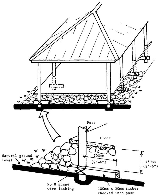
Figure 5. A method of keying timber posts into foundations
