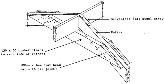
**Figure 3. Add cleats to roof structure to tie rafters together as a stable truss**
