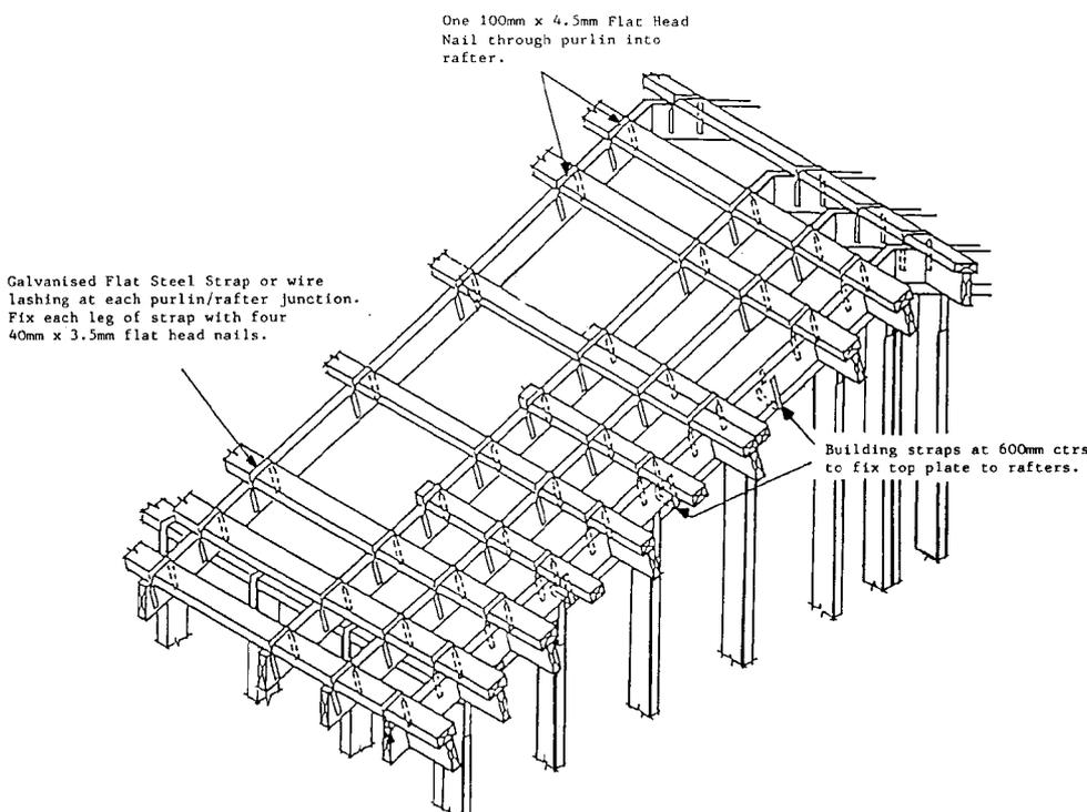
**Figure 2. Having more battens (purlins) around roof edges and tying battens to rafters wherever they cross will ensure that the roof will resist being lifted from its rafters**
