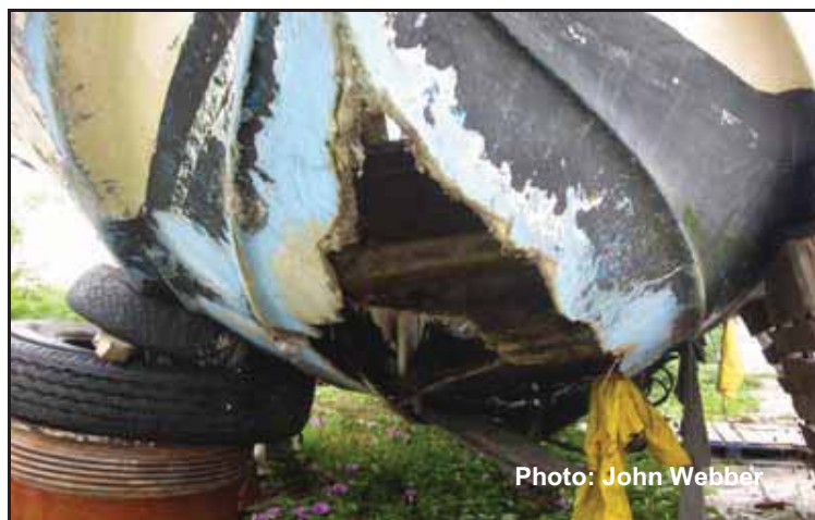
Bryson Wharf, St. John's Harbour: vessel with hull and bow severely damaged
