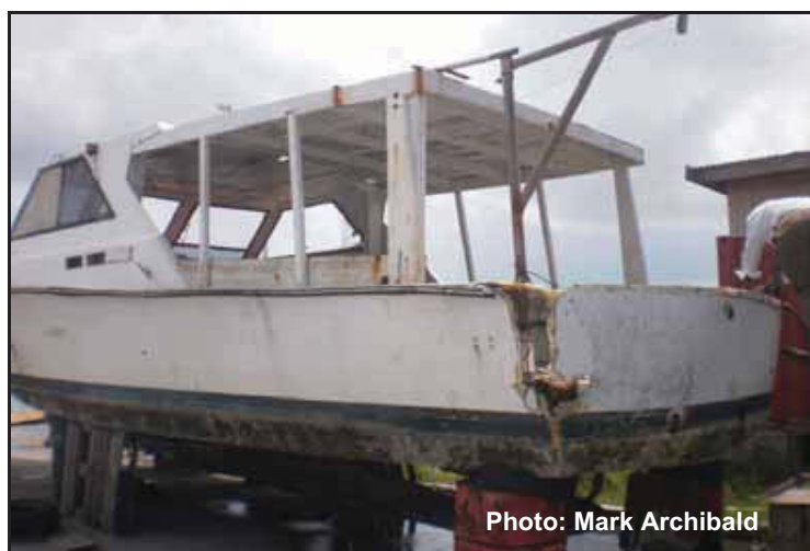
Point Wharf, St. John's Harbour: vessel with bent prop, broken keel and major damage to stern and hull
