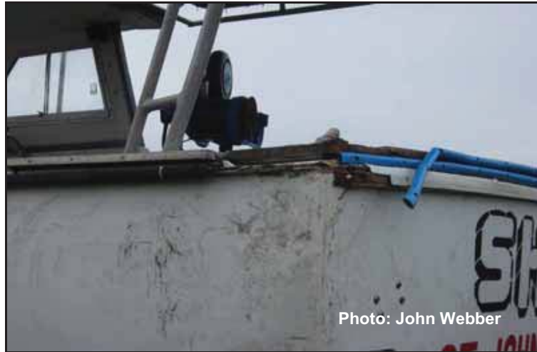
Point Wharf, St. John’s Harbour: vessel with minor damaged to gunwale
