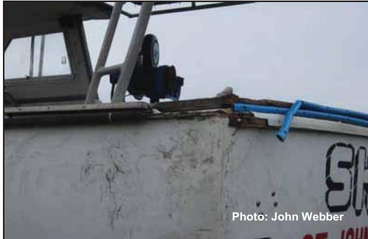
Point Wharf, St. John’s Harbour: vessel with minor damaged to gunwale
